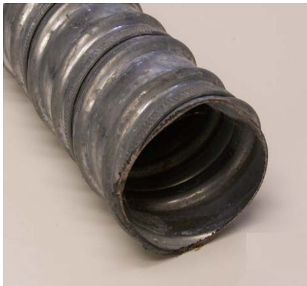
Figure 2.14: Galvanized Steel Duct
