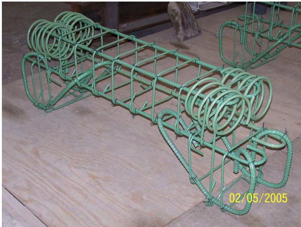
Figure 4.4: Completed Passive Reinforcement Cage
