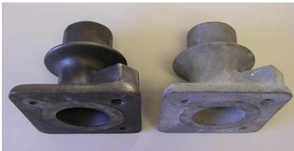
Figure 2.15: Non-Galvanized (Left) and Galvanized (Right) VSL EC5-7 Bearing Plates
